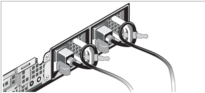
Bend the system power cables into a loop as shown in the illustration and secure the cables to the brackets using the provided strap. Plug the other end of the power cables into a grounded electrical outlet or a separate power source such as an uninterrupted power supply (UPS) or a power distribution unit (PDU).
